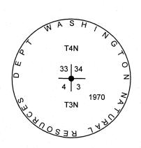
1. SECTION CORNER COMMON TO SECTIONS 3 & 4, T. 3 N., R. 9 E., AND SECTIONS 33 & 34, T. 4 N., R. 9 E. 1880- SHELTON SET A POST, 4" SQUARE, 24" ABOVE GROUND MARKED "T4NS34" ON NORTHEAST, "R9ES3" ON SOUTHEAST, "T3NS4" ON SOUTHWEST AND "S33" ON NORTHWEST FACES WITH 3 NOTCHES ON THE EAST AND WEST EDGES.
