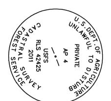
NEW REFERENCE POINT: SET 2 1/4" ALUMINUM PIPE WITH 3 1/4" USFS EMBOSSED ALUMINUM CAP S 6076'43"W, 132.27' NEW REFERENCE POINT: SET 2 1/4" ALUMINUM PIPE MTH 3 1/4" USFS EMBOSSED ALUMINUM CAP N 5875'43"E, 130.96' SET 2 1/4" ALUMINUM PIPE WITH 3 1/4" USFS EMBOSSED ALUMINUM CAP STAMPED AS SHOWN: SET 6' FIBERGLASS POST WITH A USFS 54-9 (DECAL) STICKER ATTACHED N 58E, 3' AND S 60W, 3' ON PROPERTY LINE FROM SET MONUMENT.
