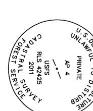
FOUND 1908 DEED (BK. "L", PG. 14) BEARING TREE: 36" FIR STUMP, N 89"W, 75.9" FOUND 1908 DEED (BK. "L", PG. 14) BEARING TREE: 36" FIR SNAG, N 90"E, 116.8" FOUND 3 1/4" USFS EMBOSSED ALUMINUM CAP AS SET IN ROS 3-456 STAMPED AS SHOWN:
