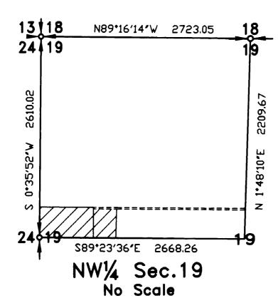
TRAVERSE STATEMENT: A closed field traverse for the parcel shown was made with a Sokkia five—second total station and related measuring equipment, all of which met State standards of WAC 332—130 at the time of this survey. Field work was conducted during the period of December 20, 2000 — January 8, 2001, the purpose of which was to monument the parcels shown.
