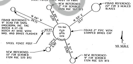
References have a Longview Fibre Co. Tag above the scribe and an 8' spike at bottom of scribe, all oriented toward the monument. Bearings to BT's taken with hand compass. Distances measured to spike.
