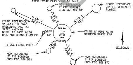
References have a Longview Fibre Co, Tag above the scribe and an 3' spike at bottom of scribe, all oriented toward the monument, Bearings to BT's taken with hard compass. Distances measured to spike,
