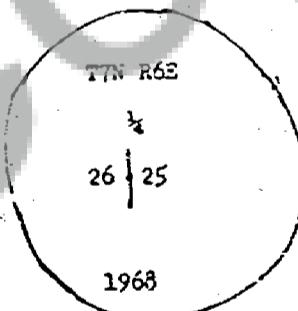
Corner: 1/4 corner common to Sections 25 and 26, T7N, R6E, W.M.
