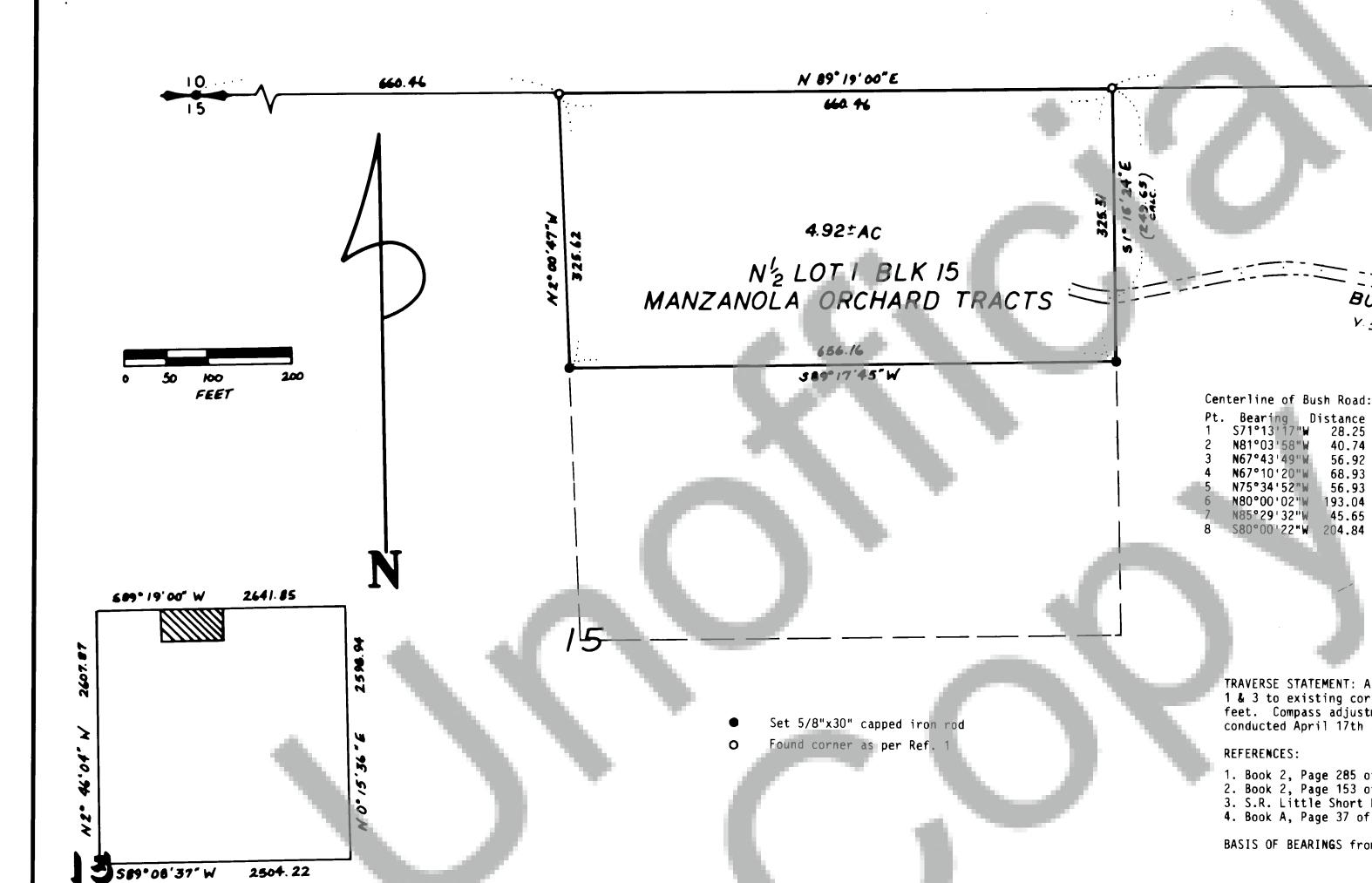
TRAVERSE STATEMENT: An open traverse was made from control in References 1 & 3 to existing corners, with a measured error of 0.19 ft. in 2115.27 feet. Compass adjustment was used to balance coordinates. Work was conducted April 17th and May 1st, 1990, and no discrepancies were noted.
